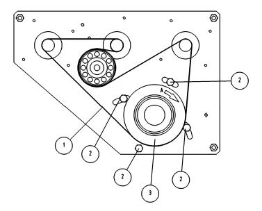
**MAG 3156 – 3306**: Transmission belt adjustment (Fig. 2) - **WARNING!!** To stretch the belt, loosen the 4 screws (2) and turn the screw (3) clockwise. To loosen the belt, turn it counterclockwise.
